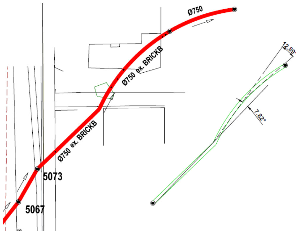
Figure 2, Alignment geometry resulting from survey work
