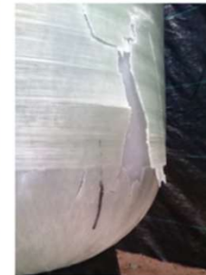
3. Implosion Tank - Partial Collapse & Broken Fiber Negative Pressure caused by siphon. No Vacuum Breaker installed. Polyethylene inner shell damaged and Fiber completely broken.
