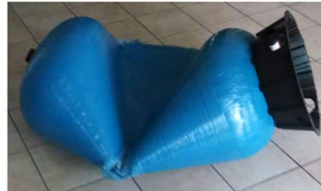
1. Implosion Tank - Total Collapse Negative Pressure caused by siphon. No Vacuum Breaker installed.
