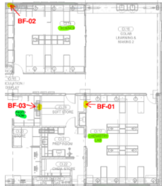
Figure 18.1: Backflow Locations (C&I Building)
