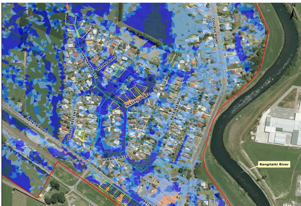
Figure 5 – Maximum Modelled Depth, Existing Pipe Network, 10-year '2090' Rainfall event, and Flooded Habitable Floors.
