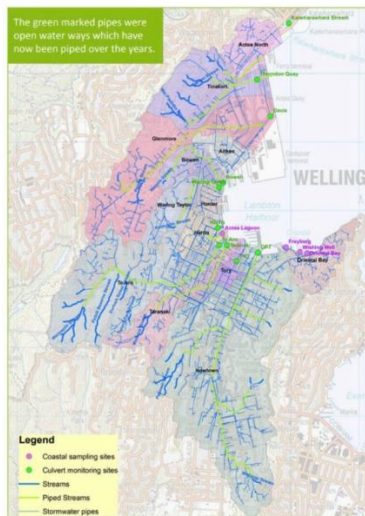
Figure 1: Piped streams in the Wellington CBD
