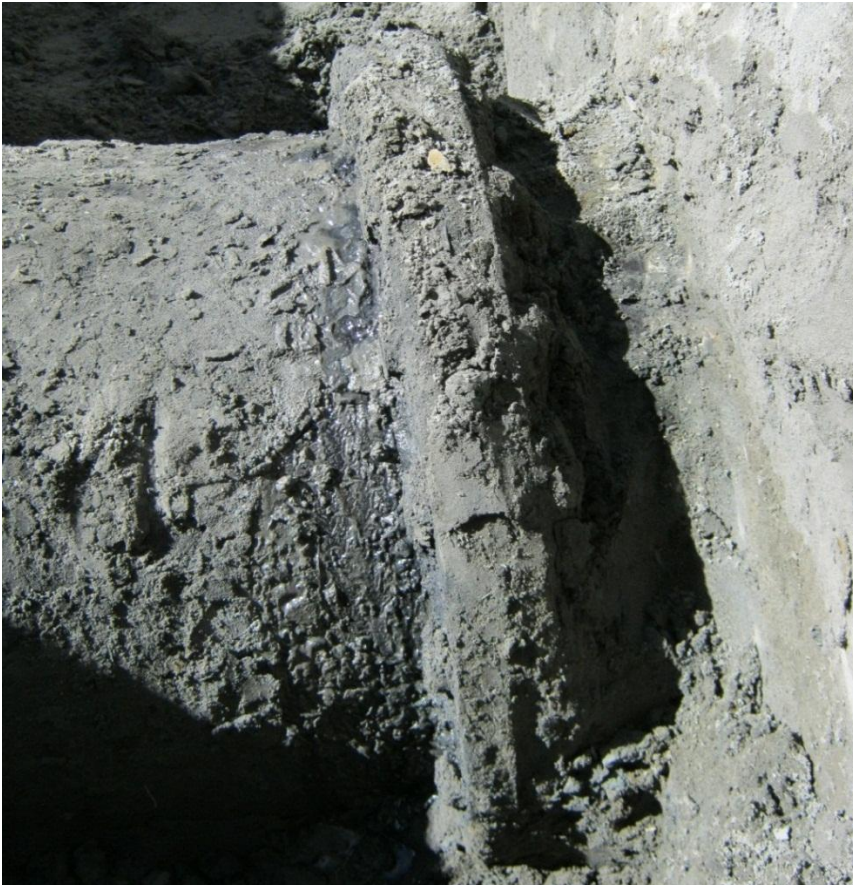
Photograph 5: Shear failure of buried cast iron pressure pipe mains at connection to valve chamber. Circumferential crack to cast iron with seeping
