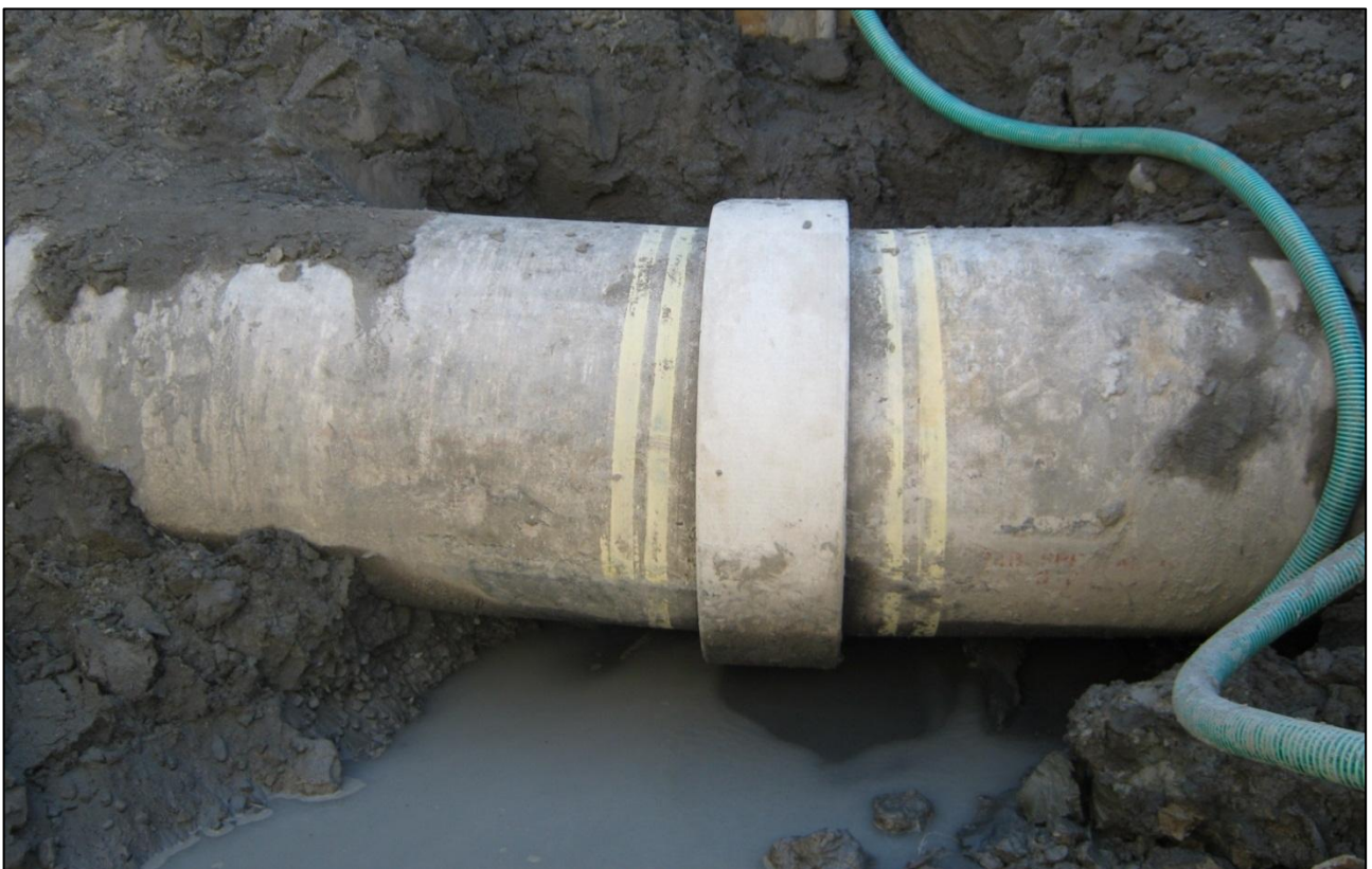
Photograph 7: Damage to asbestos cement pressure main Supertite Joint.
