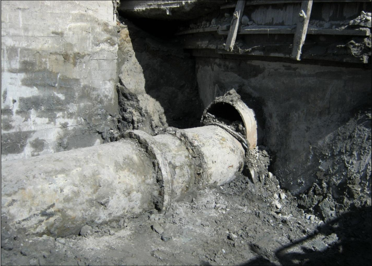
Photograph 5: Shear failure of buried cast iron pressure pipe mains at connection to valve chamber. Circumferential crack to cast iron with seeping
