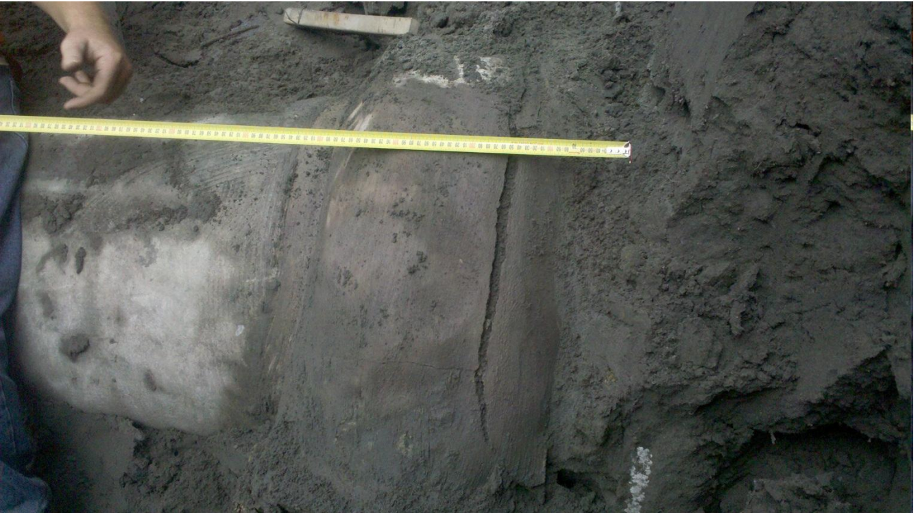
Photograph 7: Damage to asbestos cement pressure main Supertite Joint.
