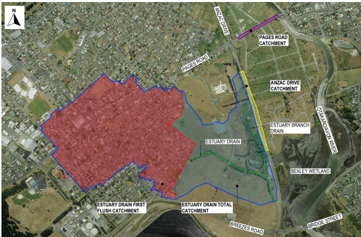
Figure 9. Existing Stormwater Catchments Draining to the Bexley Project Area
