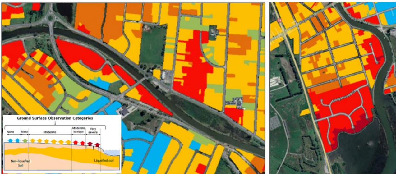
Figure 8. Severity of Liquefaction Observed at the Wainoni Project Area (left) and the Bexley Project Area (right) after the 2011 Earthquake
