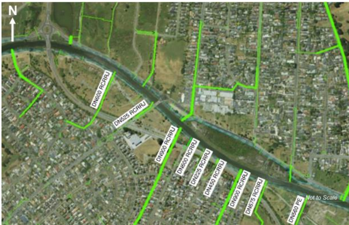
Figure 7. Existing Stormwater Pipes Located in the Wainoni Project Area
