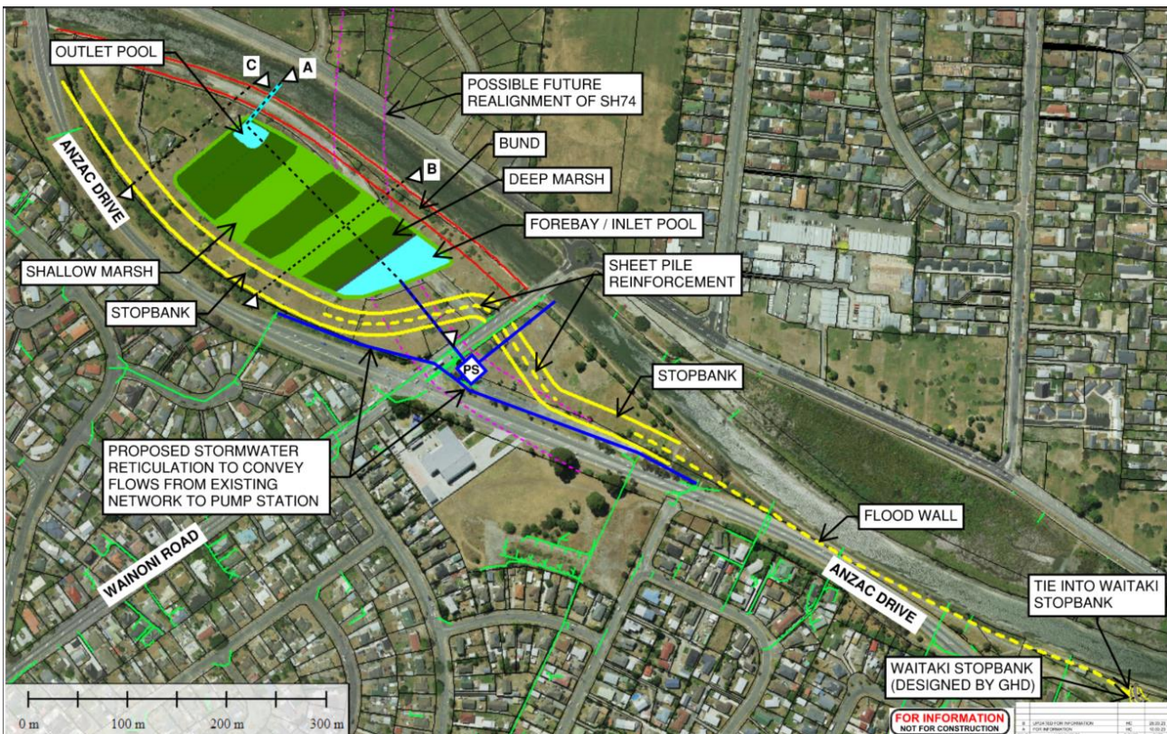
Figure 9. Schematic Plan Layout of Proposed Concept Design for the Wainoni Project Area
