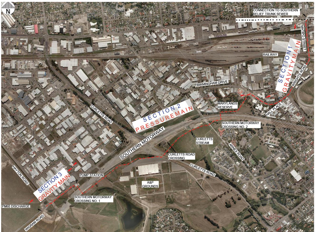
Figure 2: PM105 Pipeline Route
