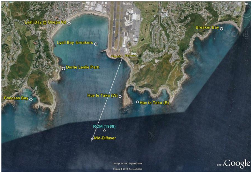
The diamond also shows location of the recording current meter (RCM) moored in 1989 for the original assessment of environmental effects investigations and used for verifying the hydrodynamic model. [Image: Google Earth and DigiGlobe]
