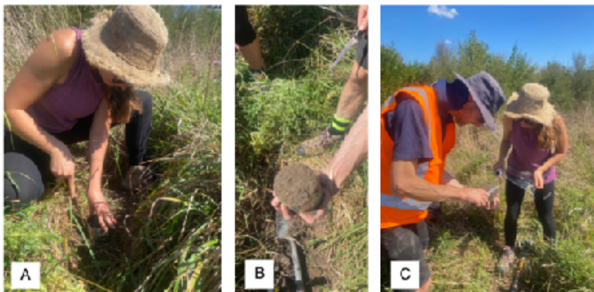
Figure 5: Soil coring process. (A) digging the core into the soil with the help of a serrated knife. (B) the soil core, just removed from the ground. (C) wrapping the core for safe transport and storage.
