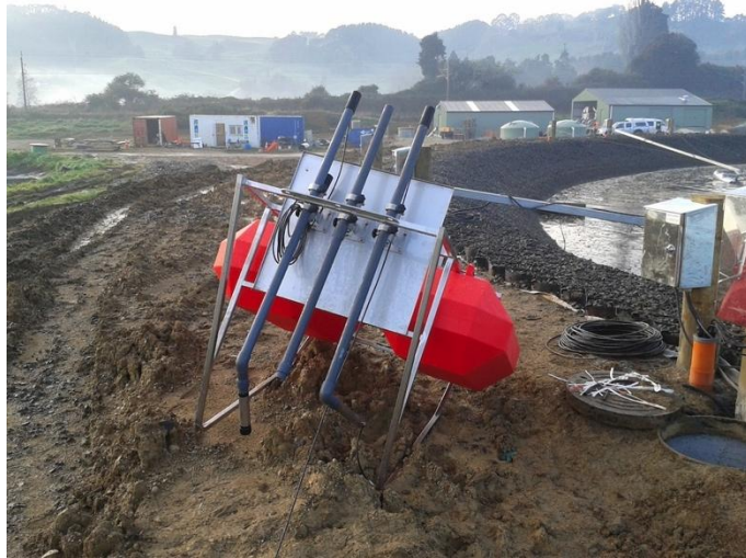
Photograph 8: On-line Probes Mounted on Float
