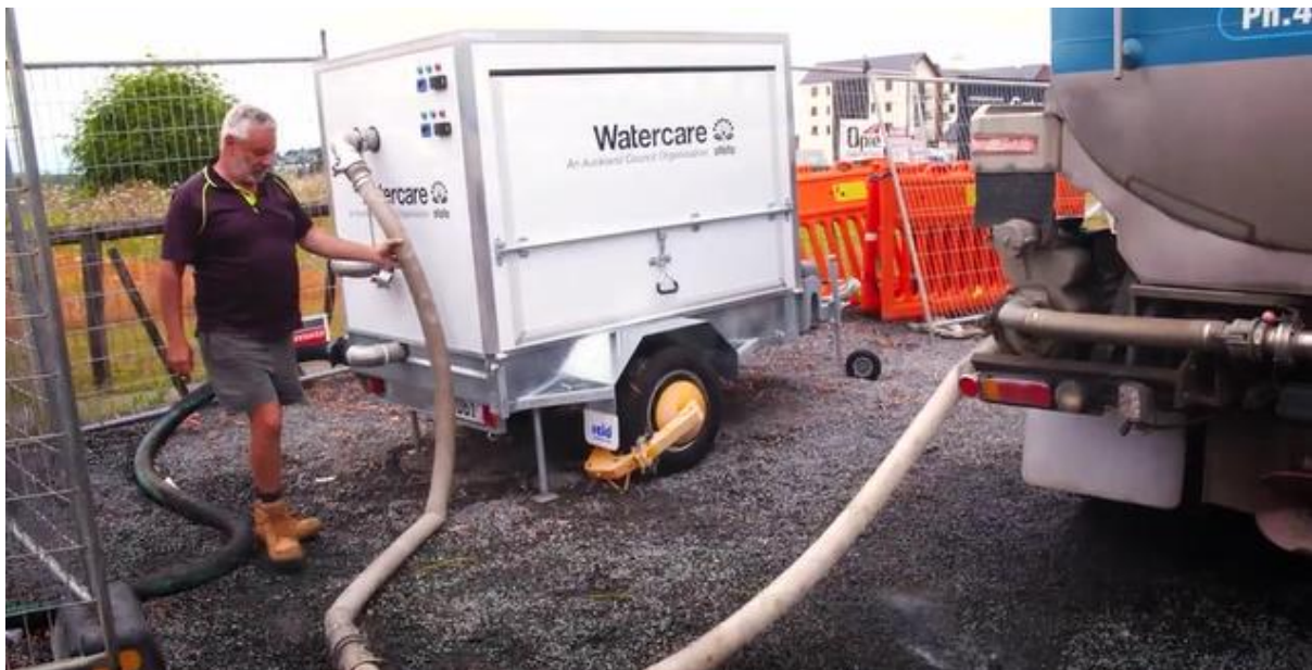
Photograph 1: A prototype of the portable tanker filling station.
