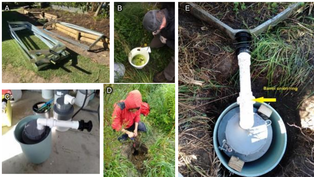
Figure 6: Set up of the runoff collectors. A) Frames of the collectors as they were built. The frames were dug 5cm into the soil, with the triangular end leading to the sample inlet oriented downhill. B) Original collection system did not allow for maintaining a "clean" sample. C) New system prototype, which is better sealed and included a filter to impede the intrusion of litter and animals. D) Set up of the new collectors in the field. E) The new system established in the field.
