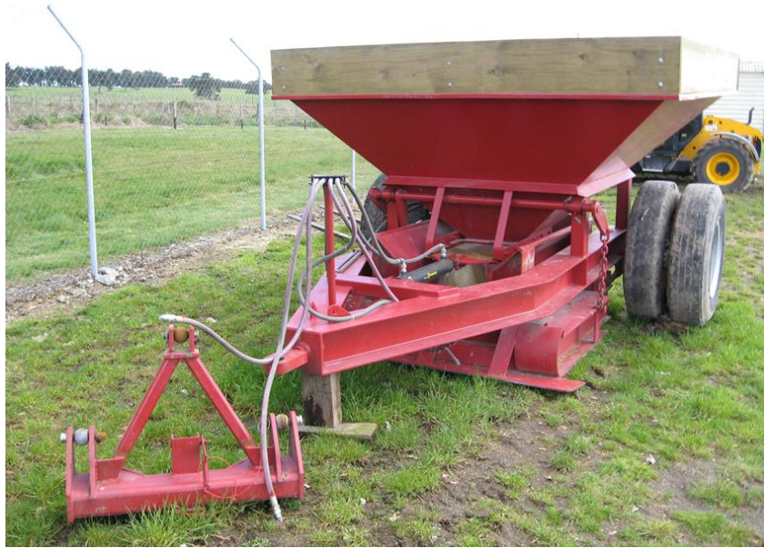
Photograph 1: Rut Filler Trailer specifically designed by TDC
