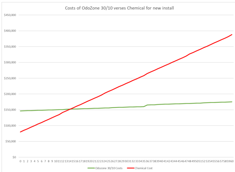
Figure 6: OdoZone verses chemical dosing over 60 months
