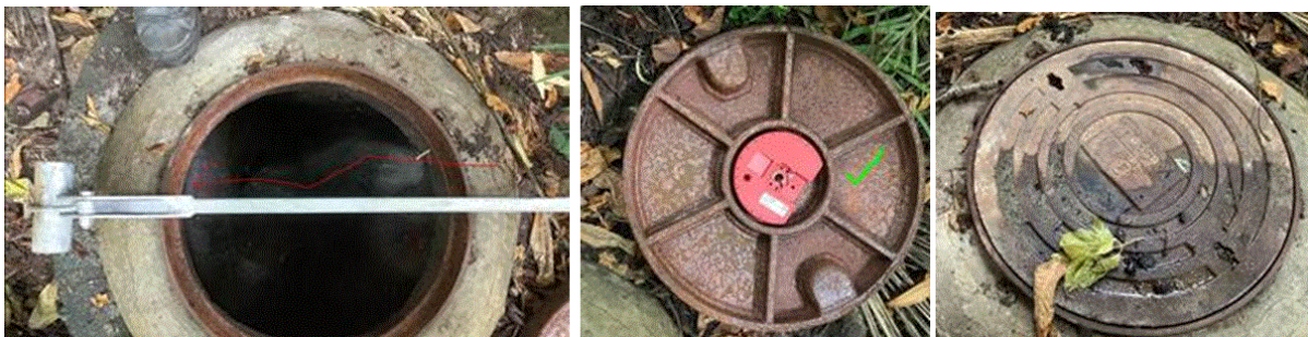
Figure 4: Example 2 from preliminary site survey: photos showing, from left to right, alignment of channel, sensor placement, manhole surface
