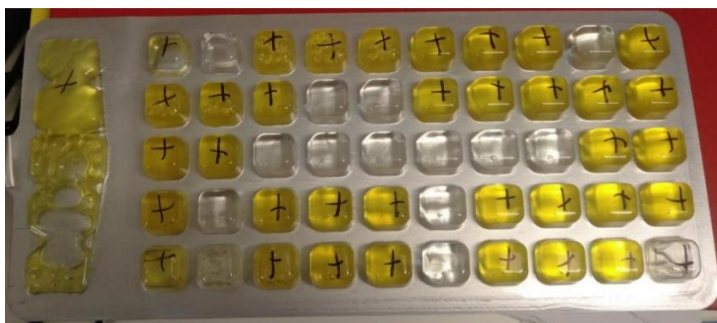
Figure 3: Colilert tray with yellow wells indicating Total Coliforms and clear wells no total coliforms. The yellow wells when exposed to UV light then fluoresce if E. coli are present.
