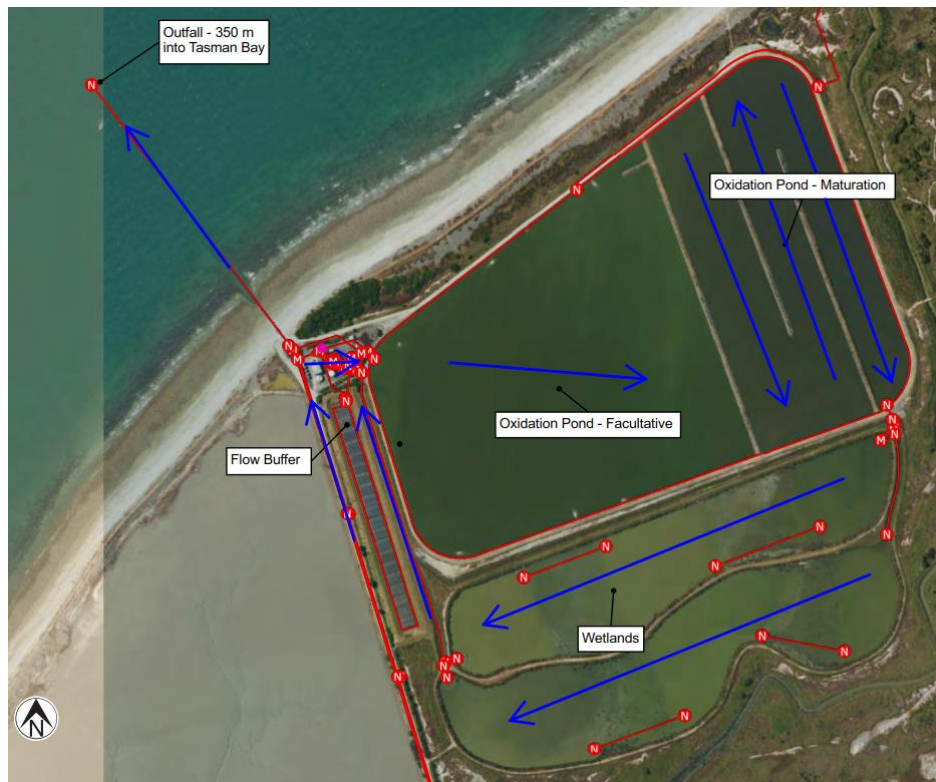
Figure 1: Overall plan of NWWTP with typical flow path shown in blue (Source: Top of the South Maps (TOTSM)).
