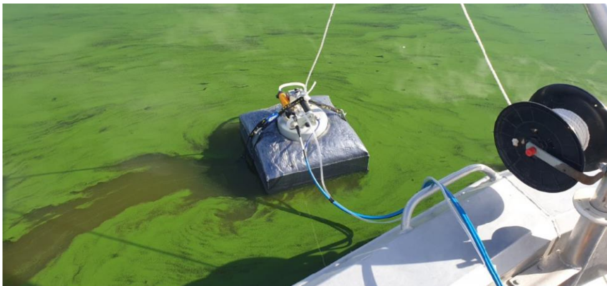
Photograph 2: West System accumulation chamber in place to capture emissions measurements at NWWTP. A silver float surrounds the accumulation chamber. (Source Di Elliot).
