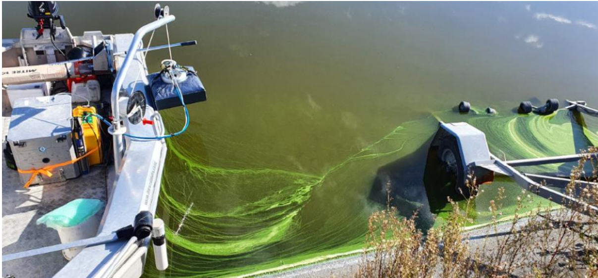
Photograph 5: Photo of boat setup prior to sampling. Note accumulation chamber lifted clear of water with crane. Source: Di Elliot.
