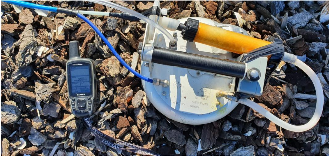
Photograph 3: Accumulation chamber in place sampling biofilter emissions. Source: Di Elliot.
