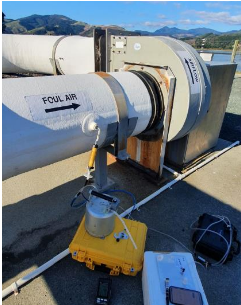
Photograph 4: Direct sampling of gaseous concentration from foul air duct. Source: Di Elliot.
