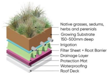
Figure 3: Semi-Intensive Living Roof Typology
