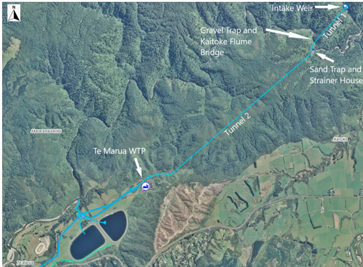
Figure 2 Te Mārua Raw Water Intake
