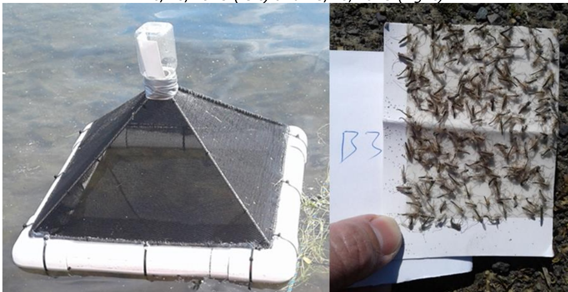
Figure 12: Left: an emergence trap used on the FEC. Right: a sticky card from the apex of a trap with adult midges stuck to it. Photos taken by the author on 26/10/2018 (left) and 15/10/2018 (right).
