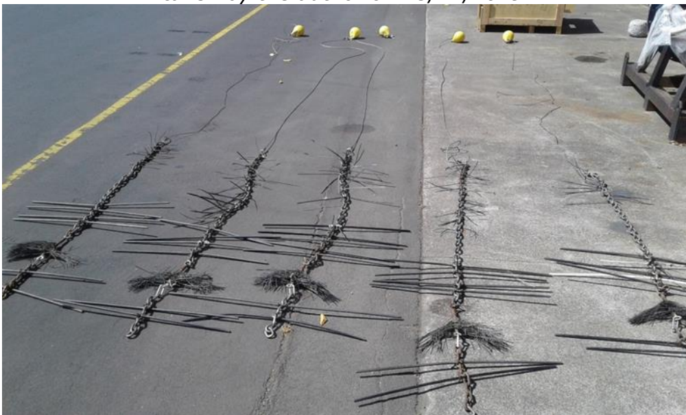
Figure 7: Modified chains version 2 with nylon rods attached as spikes. Photo taken by the author on 13/12/2019.
