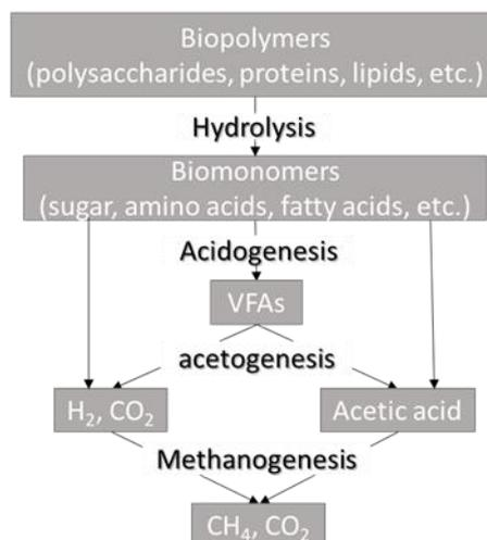
Figure 1 Anaerobic digestion process
