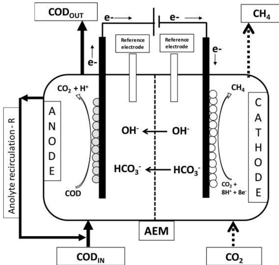
Figure 2 MEC reactions (adapted from Zeppilli et al., 2019)
