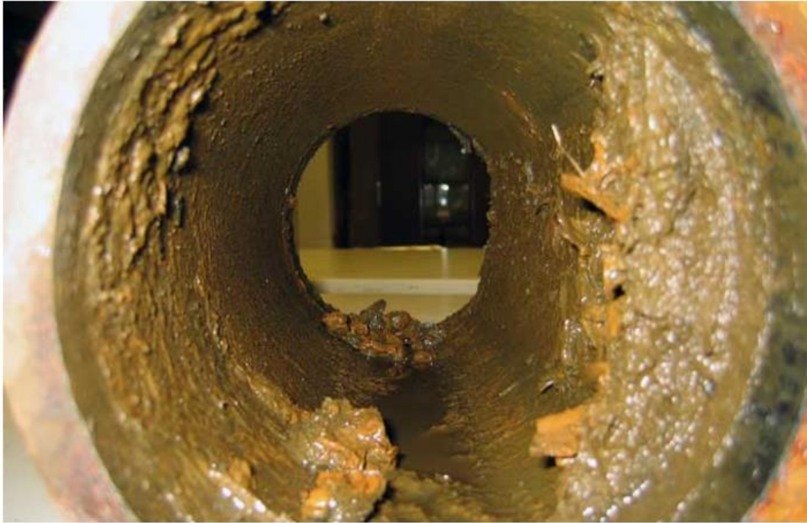
Photograph 2: Iron Pipe Cross Section showing Biofilm
