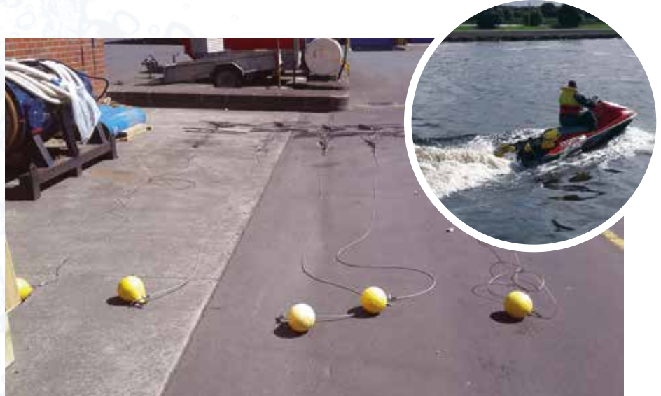
World-first 'lawn mowing' approach to pest control involves a jet ski pulling multiple chains with spikes through the 17-hectare treated wastewater channel near Watercare's Māngere Wastewater Treatment Plant.
