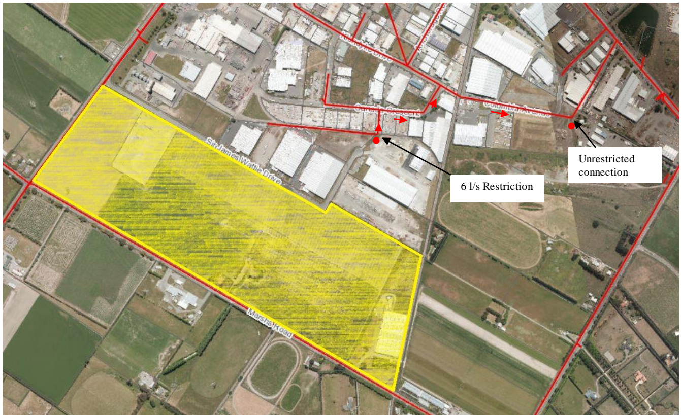
Figure 1: Site location with location of sewer restrictions
