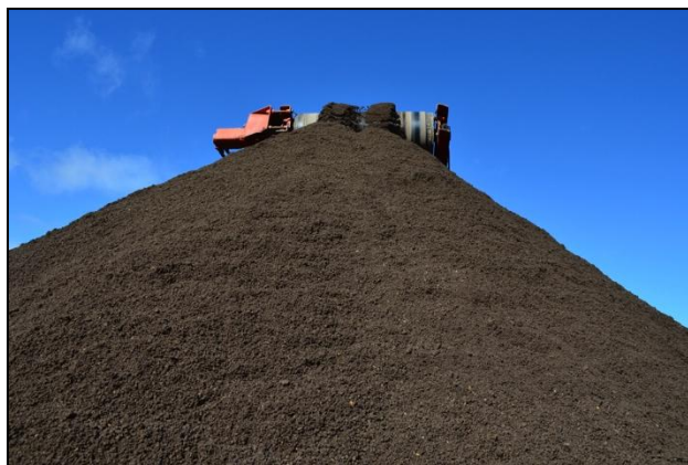
Photograph 3: Screened (5 mm) MyNOKE® organic Wormicast produced from pulp mill solids coming off a conveyor.
