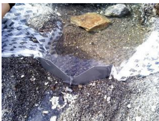
Photo 5: A temporary weir deployed at Taharepa Bath warm spring.
