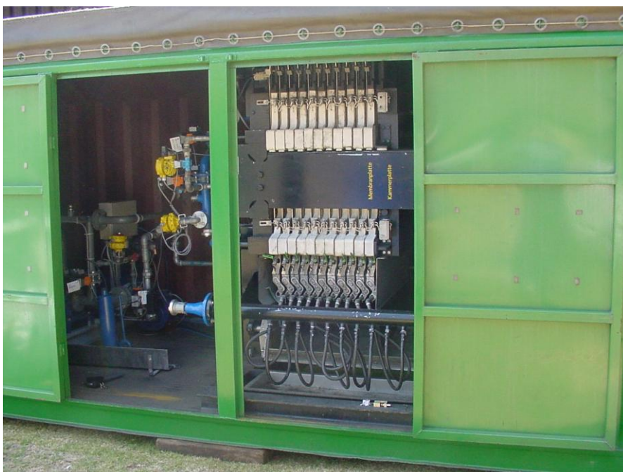
Photograph 3: The Ishigaki filter press trial unit.
