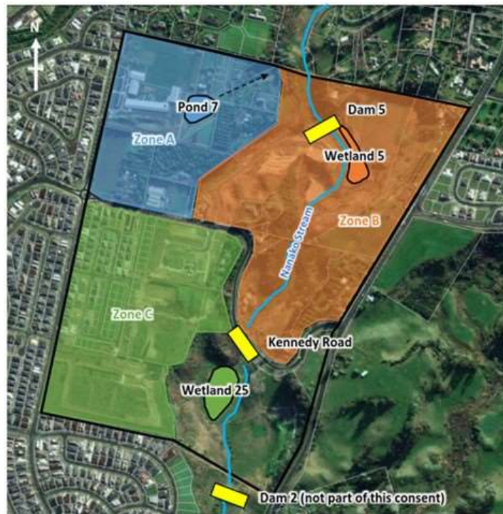
Figure 10: Location of stormwater management devices
