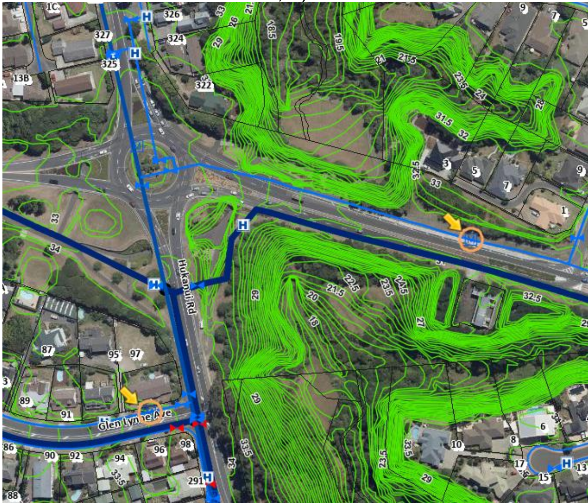
Figure 14: GIS map of water network showing two meters (circled) with an elevation difference of 2 metres, yet 5 metres difference in head
