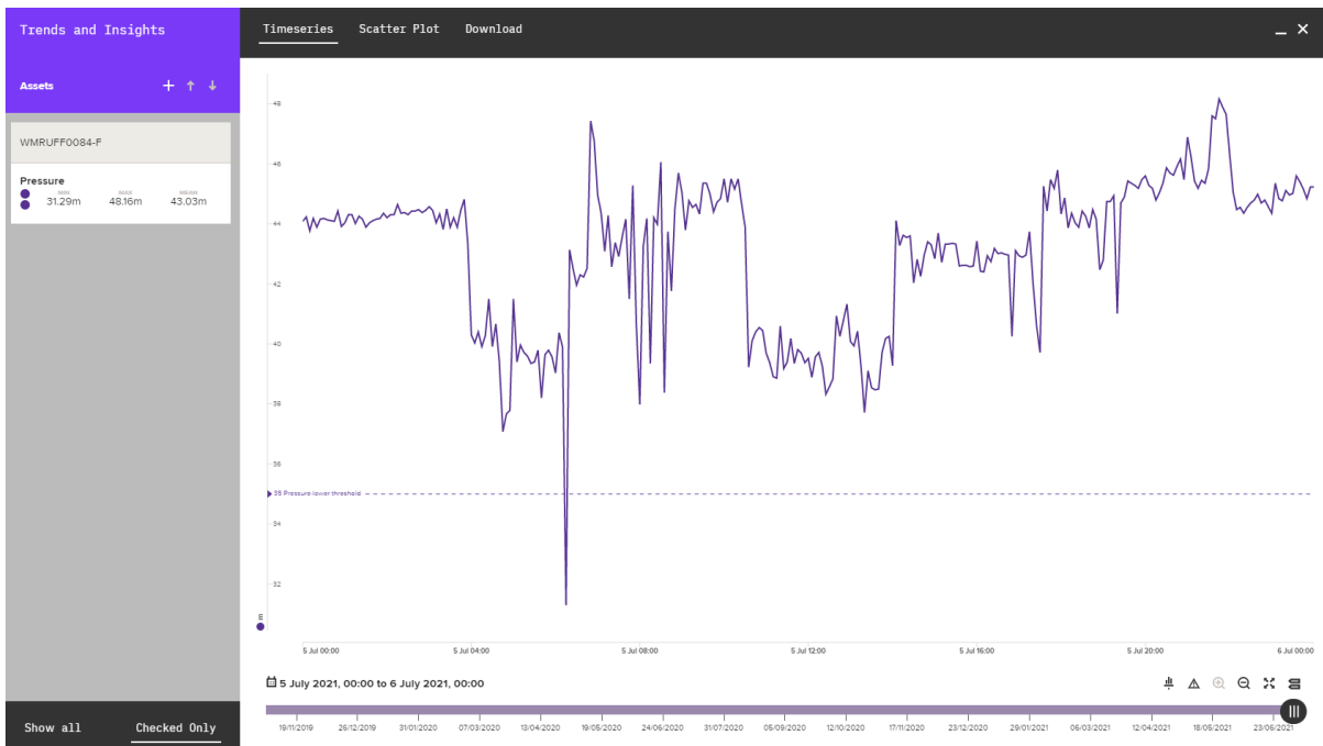
Figure 10: Example of pressure dropping below the (dotted line) threshold, which would trigger an alarm
