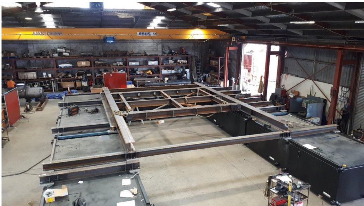
Photograph 9 - Steel spreader frame
