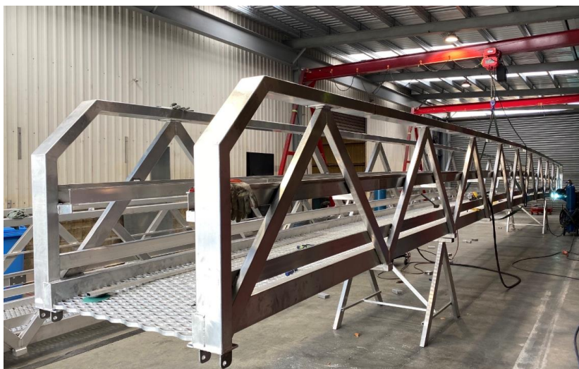
Photograph 3 - Gangway during manufacturing process
