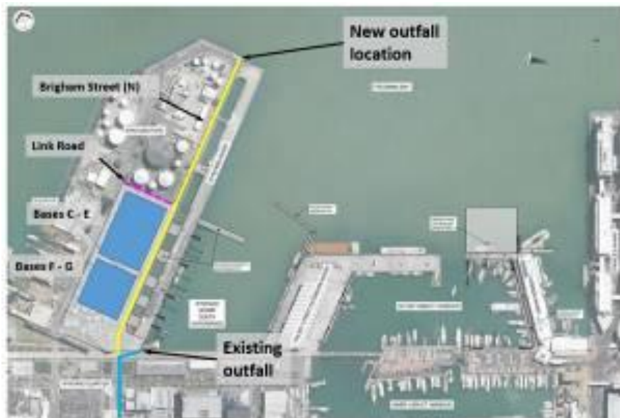
Figure 1 – extension of Daldy Street Outfall
