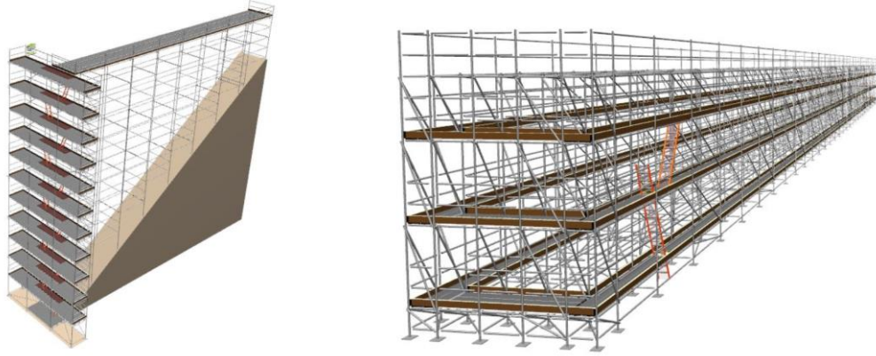
Figure 6: Proposed Scaffolding Visualisation for Original Tender Scope showing the extent of the works required on the river banks.
