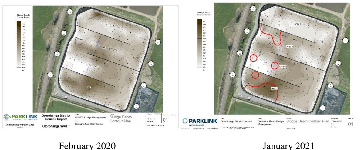
Figure 4 – Pond sludge depth contours prior to and after AMD dosing in the denitrification (top) zone.
