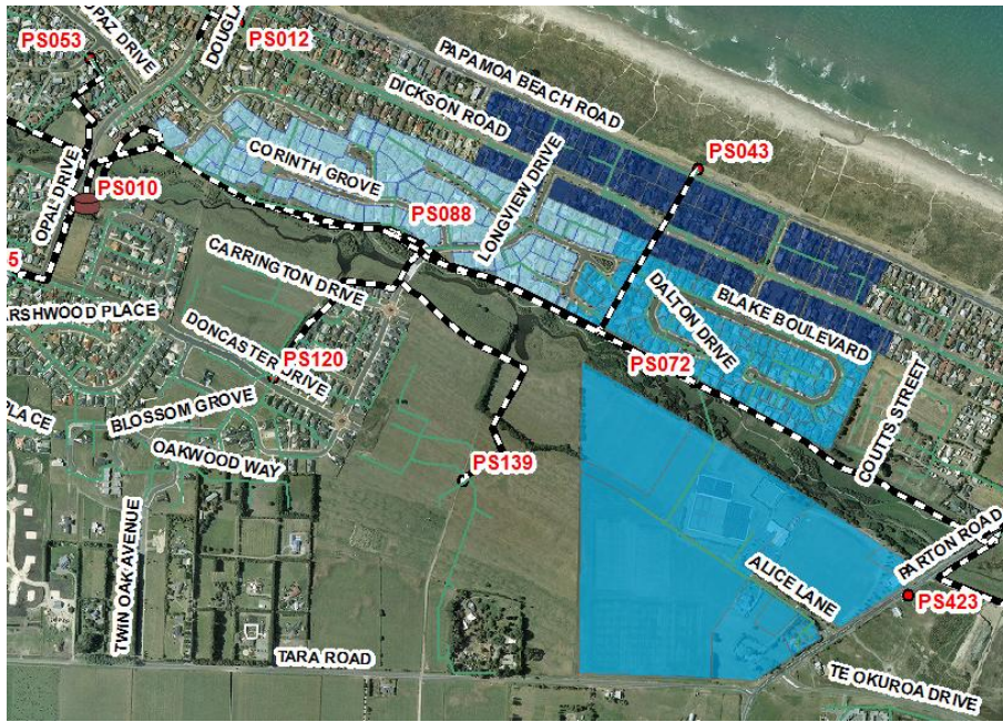
Figure 11: Opal Drive pressure system, a complex injection system in Papamoa network
