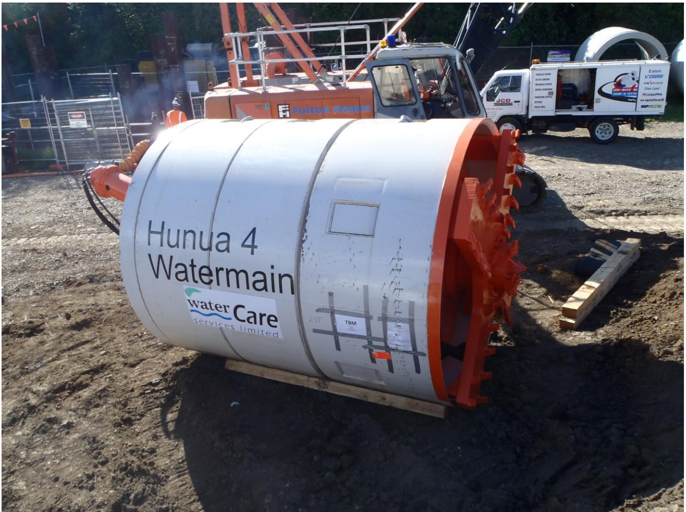
Photograph 1: SH1 Crossing 2.75 m diameter EPB TBM
