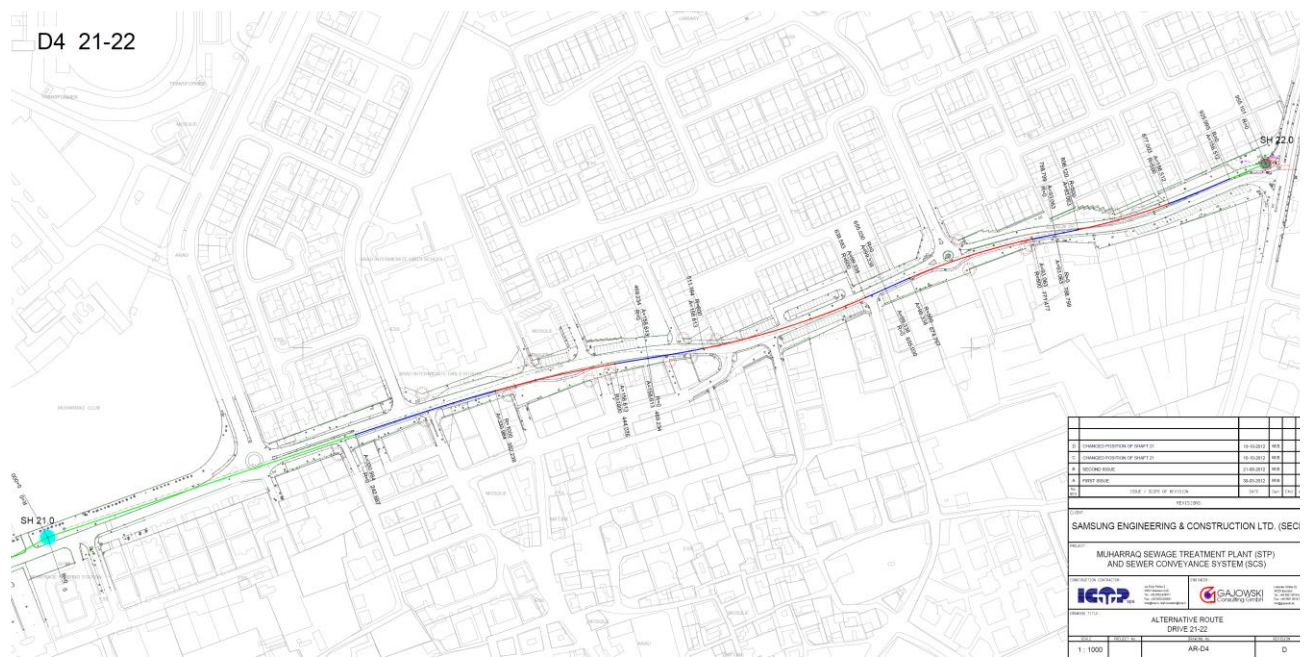
Figure 3. Post Engineering/Optimization of Pipeline Route along Fort Arad area (PS B2 to PS)
