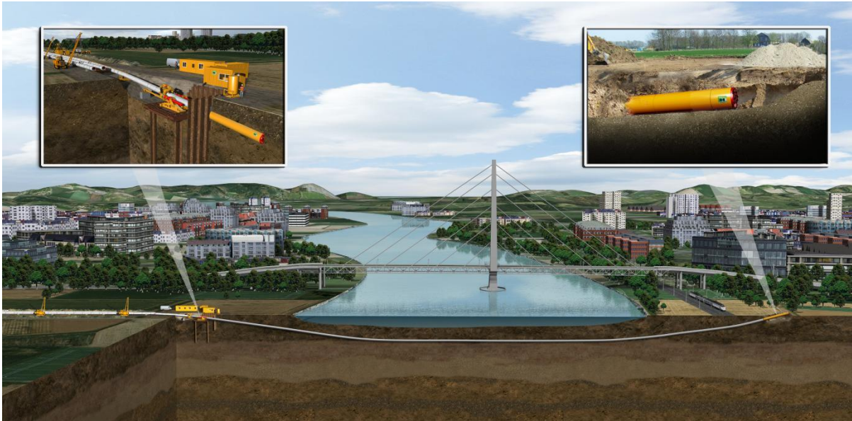
Figure 1: River crossing using the Direct Pipe method from left to right
