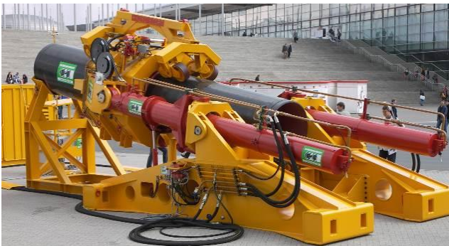
Figure 3: The Pipe Thruster HK500PT exhibited at the Hannover Fair in 2006 clamping a 48" steel pipe.
