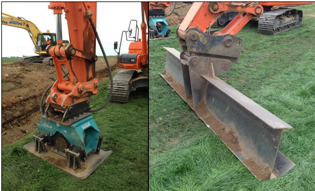
Figure 5: Excavator mounted vibration compactor & backfill tool
