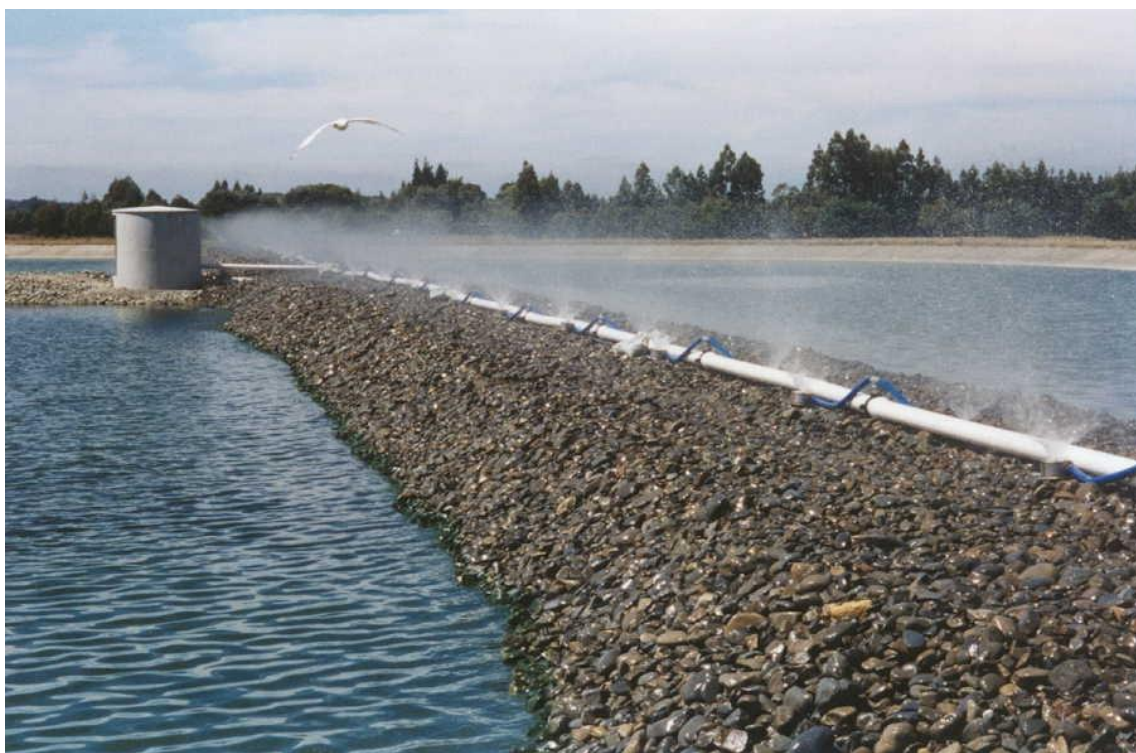
Figure 2 – Pond effluent being sprayed over internal rock baffles at Rangiora WWTP (from 2003 to 2006)
