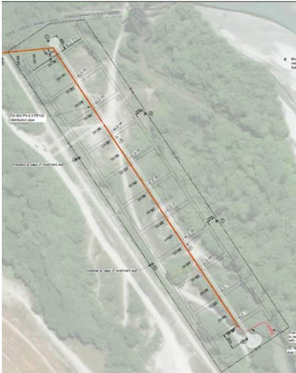
Figure 2: Plan view of the eleven DAD dispersal fields with 800 mm distribution pipe shown in red in centre
