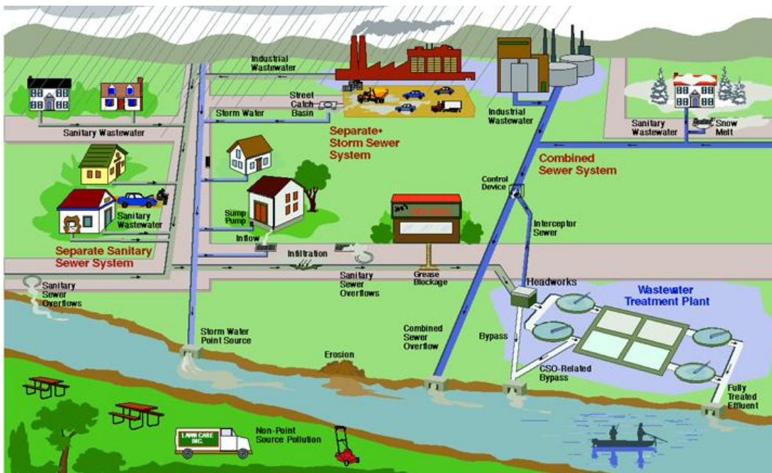
Figure 2: Typical stormwater and wastewater system schematic (EPA, 2015)
