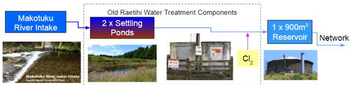
Figure 1: Main Components of Raetihi WTP 2013
