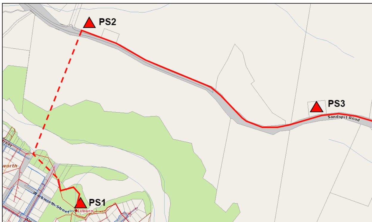
Figure 6: Map of reference design pump station locations and Mahurangi River Crossing alignment.
