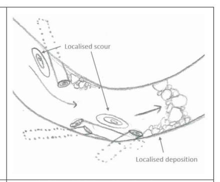
Example of woody debris placed within a stream channel and the predicted areas of scour and deposition which are critical to aquatic habitat.
