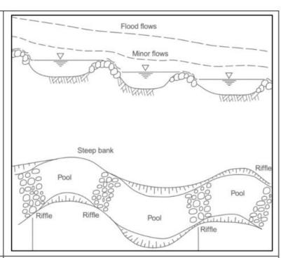
Plan and cross section view of riffle construction and placement in regard to meanders and flows (image from Brisbane City Council, 2003).
