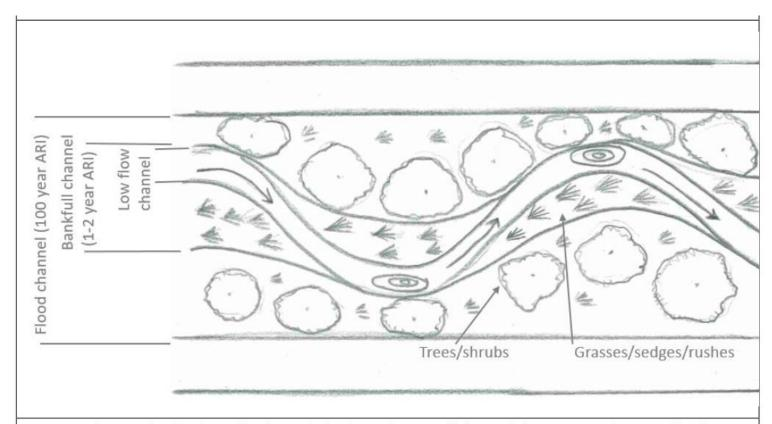
Conceptual example of a desirable channel planform showing all channel elements in relation to flood capacity, as well as indicative planting for habitat and conveyance.
