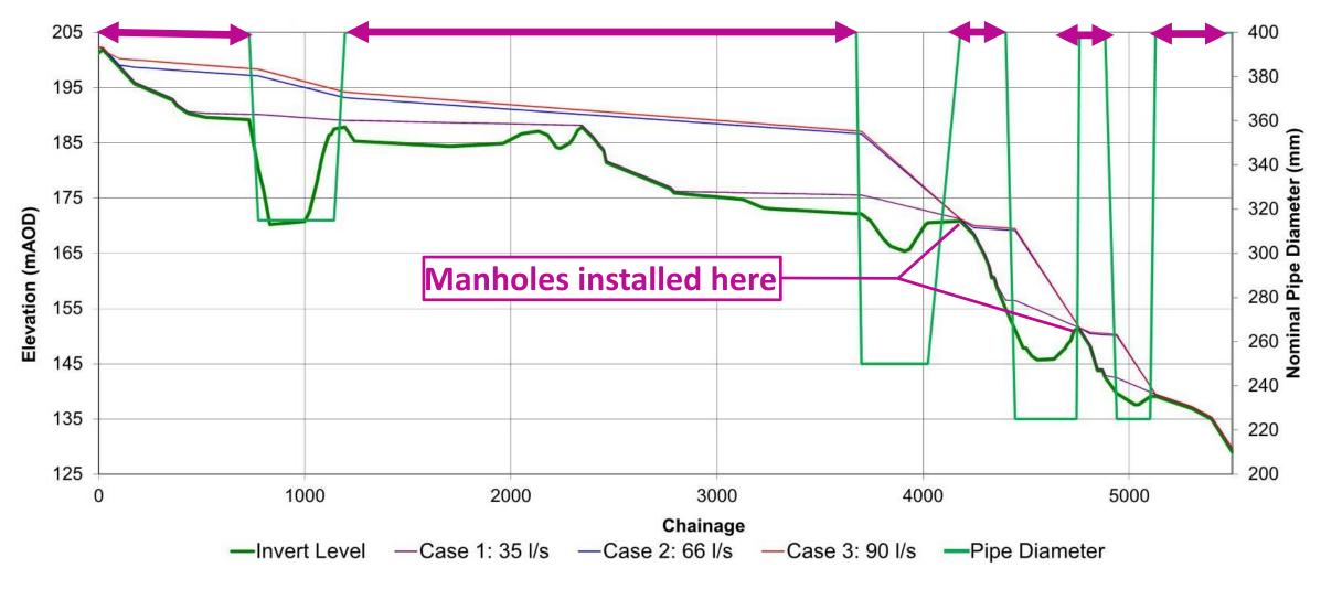
Diameter in gravity sections allows for part full flow and manage air more effectively
