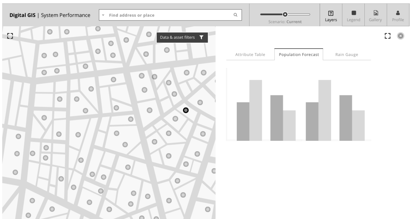
Figure 11 – Clickable wire-frames help test user interface concepts with users without having to invest in costly development changes
