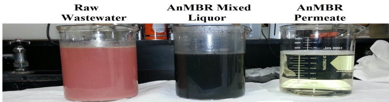
Photograph 2: Example of the effluent (permeate) quality available from an anaerobic MBR system.
