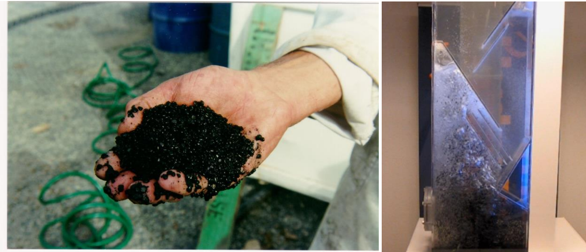
Photograph 3 and 4: A handful of granular sludge, and a representation of the gas solids separator in a high rate reactor.
