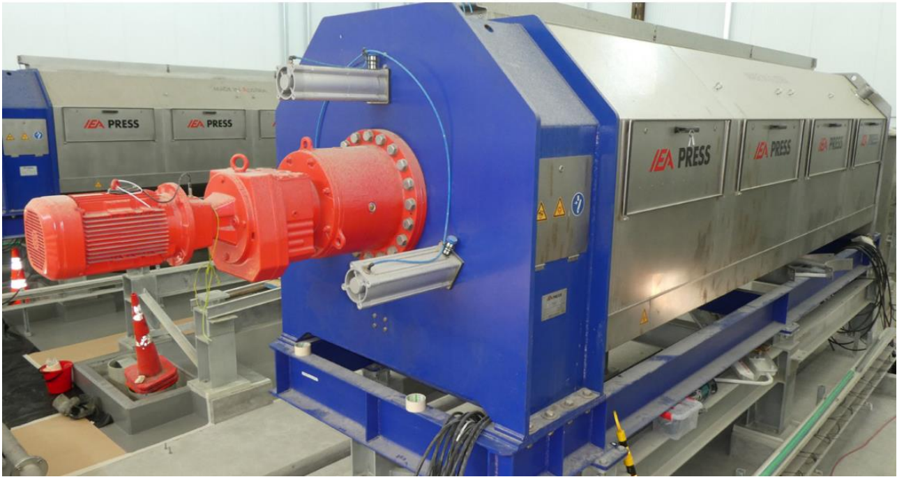
Photograph 4: Full scale screw presses
