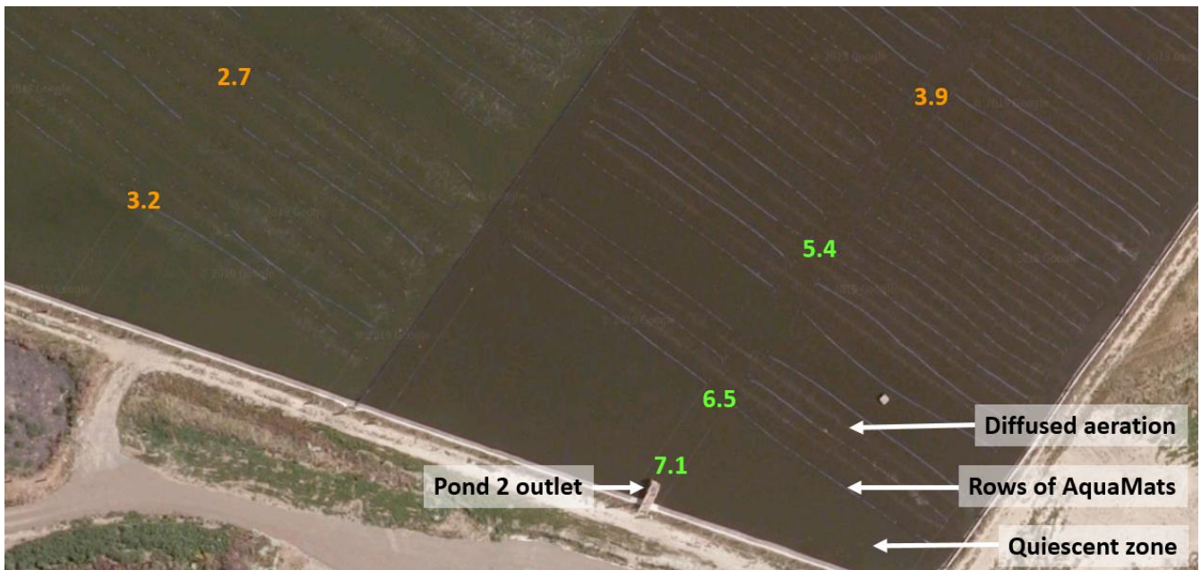
Figure 10: Surface DO (mg/L) at Matamata WwTP, April 2019
